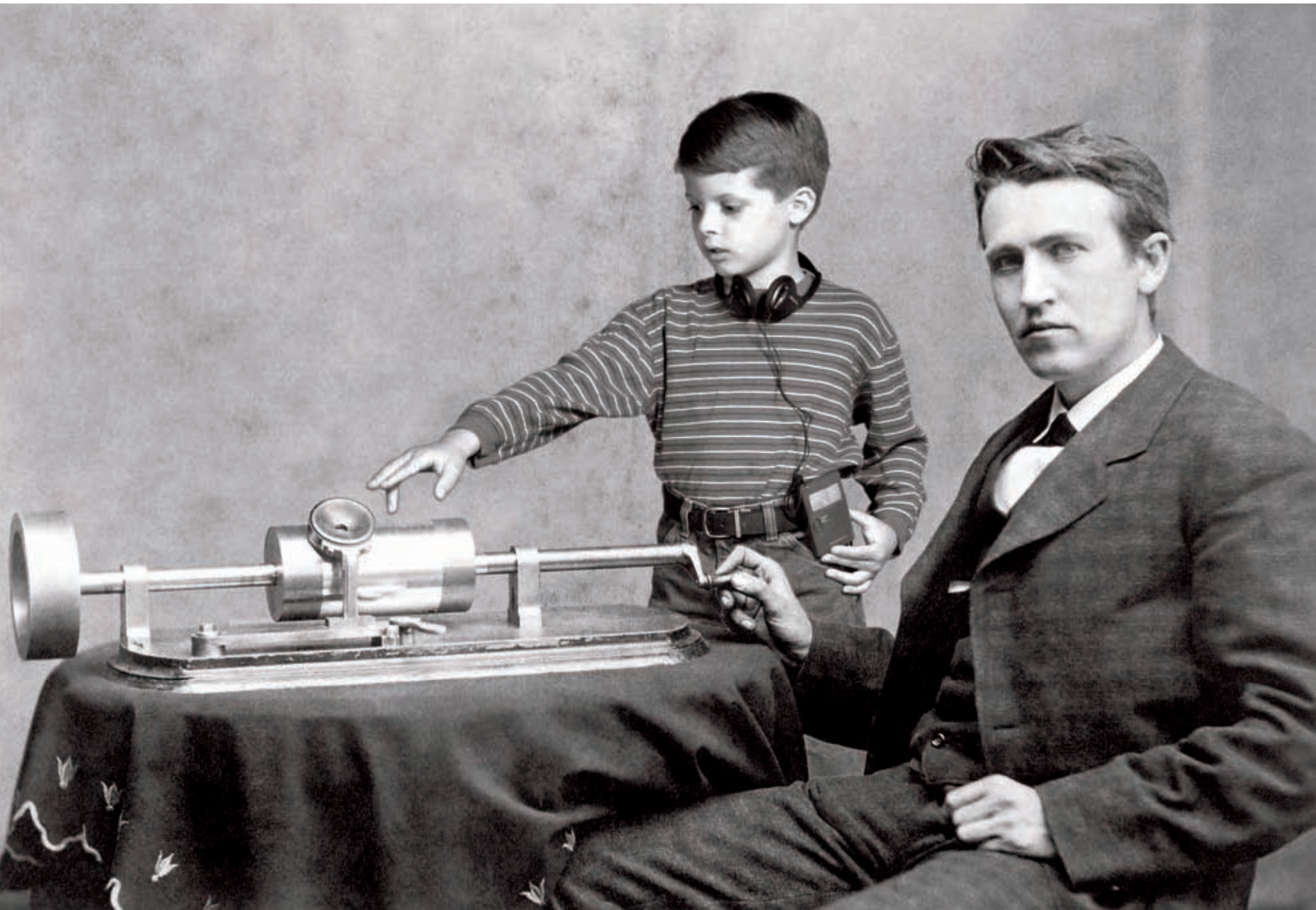
THOMAS EDISON DEMONSTRATES HIS TINFOIL PHONOGRAPH. Location: The Washington, D.C., portrait studio of photographer Mathew Brady. Date: 4/18/1878. Visible: The phonograph's hand crank, cylinder, and recording stylus mechanism. © Bettmann/CORBIS
